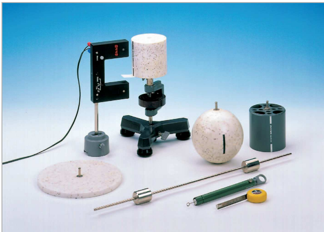
Fig. 1: Experimental set-up for determining moments of inertia of various bodies.
