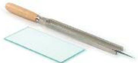
For recording low-frequency vibrations on a glass plate coated with soot; 128-Hz tuning fork with wooden handle, complete with stylus; total length (without stylus tip): approx. 295 mm; glass plate 120 x 50 mm included
