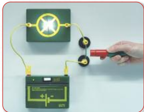
Experiment: Model of a Reed relay - contactor (make-contact) closed by means of a bar magnet
