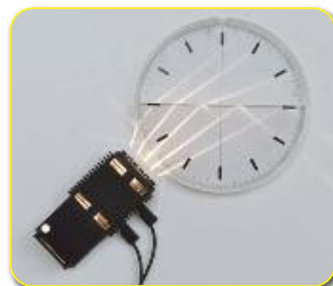
Experiment: Light ray refraction phenomena when passing from water to air at various angles
