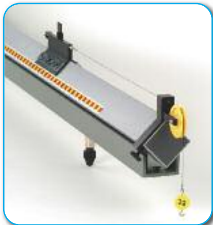
Detail: Pulley for deflecting force and weight driving glider (experiment: uniformly accelerated motion)
