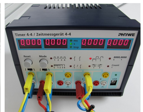
Fig. 7: Connection of the light barriers and the starter system
