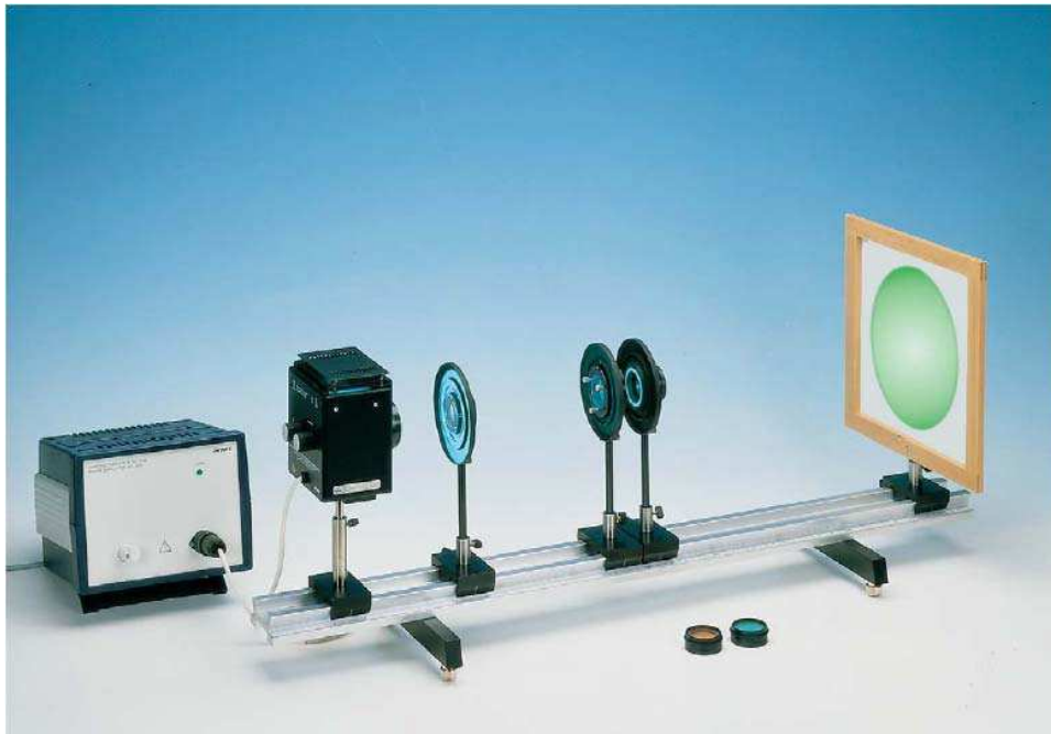
Fig. 1: Experimental set-up for determining wavelength using the Newton's apparatus.
