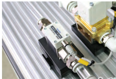
▲ Flow rate sensor, Proportional control valve
