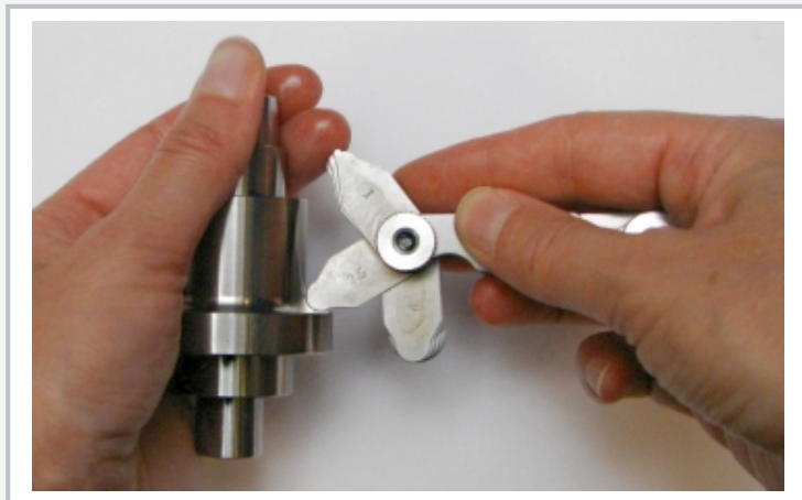
Measurement of radius using a convex radius gauge
