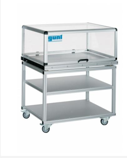
The illustration shows PT 500.01 together with the base plate with protective hood from the base unit PT 500.
