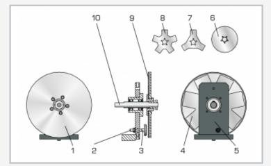
1 guard disk, 2 adjuster screw for gap between magnet and blades, 3 permanent magnet, 4 fan rotor with 7 blades, 5 bearing block, 6 mass disk to simulate axial forces, 7 fan rotor with 3 blades, 8 fan rotor with 5 blades, 9 fan blade, 10 fan shaft
