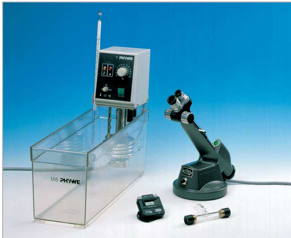
Fig. 1: Experimental set-up for measuring the rotation of sugar solutions.
