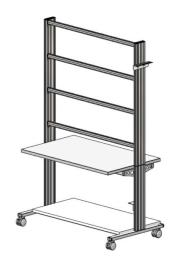
> For attachment to left or right, fastening materials included > Acid-resistant epoxy-resin powder coating of thickness 80  $\mu m$  approx., colour RAL 7047
