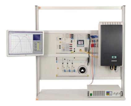
EPH 3.2 Configuration of photovoltaic systems to operate in parallel with the power grid
