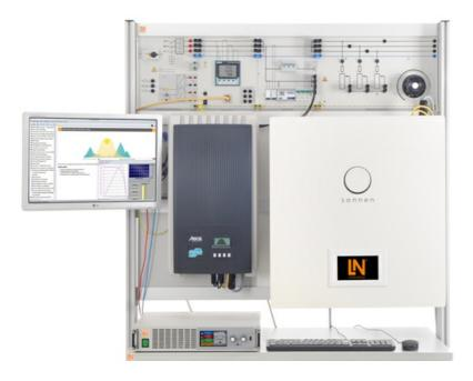
EPH 3.4 Investigation of battery storage units in conjunction with photovoltaic systems
