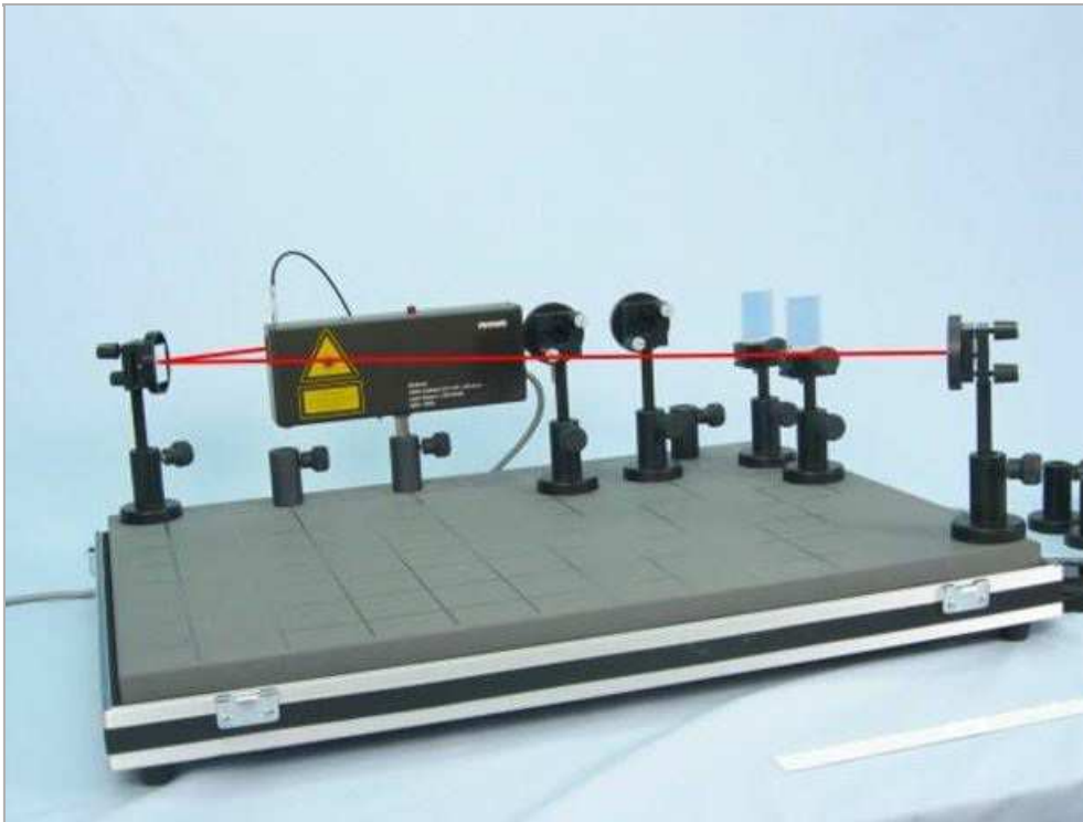
Fig. 6: Adjusting the mirrors M2, M3, M4 and the beam splitters BS1, BS2.
