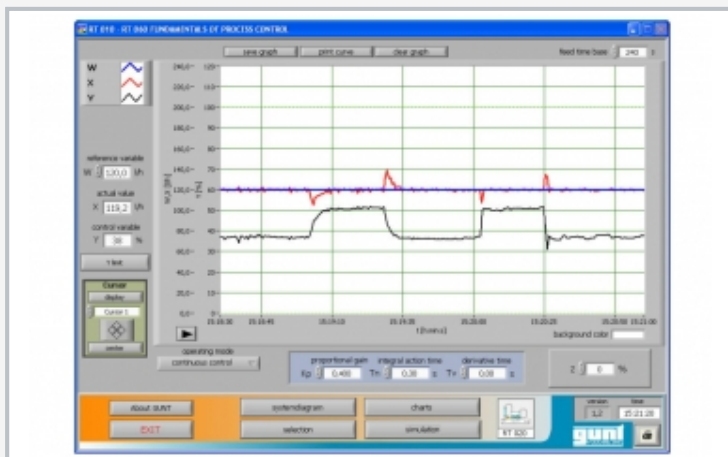
Software screenshot: flow control, controller with PI response with different values for K_p and T_i , introduction of a disturbance variable
