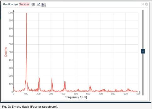
Use the FFT analysis and determine the position of the resonance frequency of the 1000 ml flask, which is only filled with air, from the spectrum.
