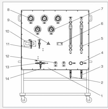
1 panel, 2 hot water feed, 3 cold water feed, 4 pressure reducing valve, 5 rotameter, 6 bracket for standard fitting, 7 Bourdon gauge, 8 thermometer, 9 flushing valve connection, 10 adjustable centre distance, 11 wall fitting connection, 12 standard fitting connection, 13 mixed water connection, 14 mixed water drain
