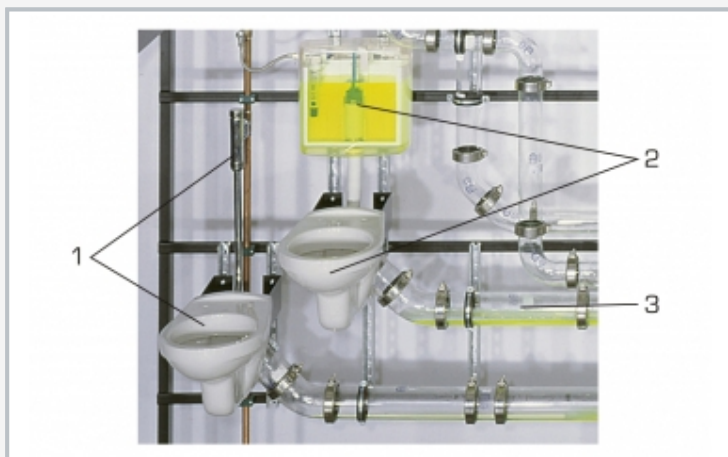
1 toilet bowl pressure flush, 2 toilet bowl with cistern, 3 transparent pipes
