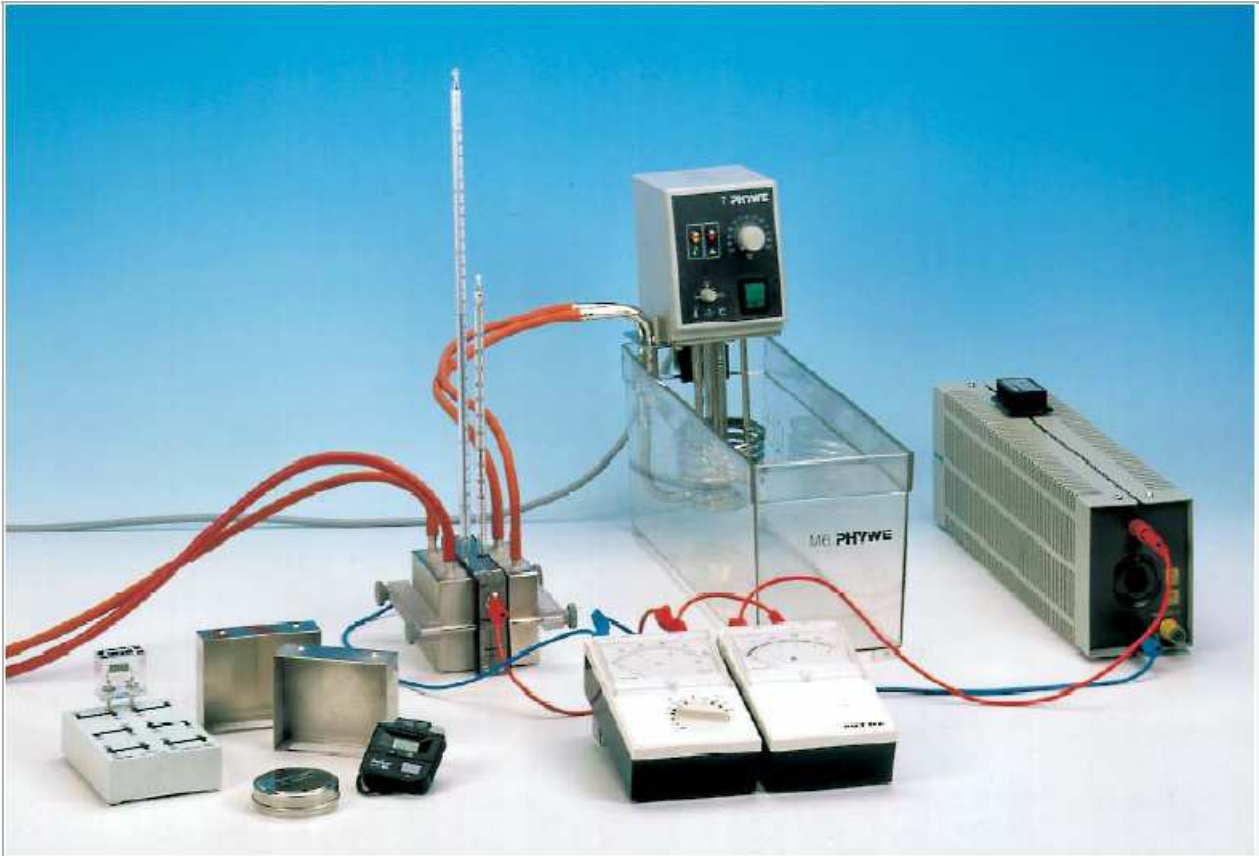
Fig. 1: Experimental set-up for measuring no-load voltage and short-circuit current as a function of temperature difference.
