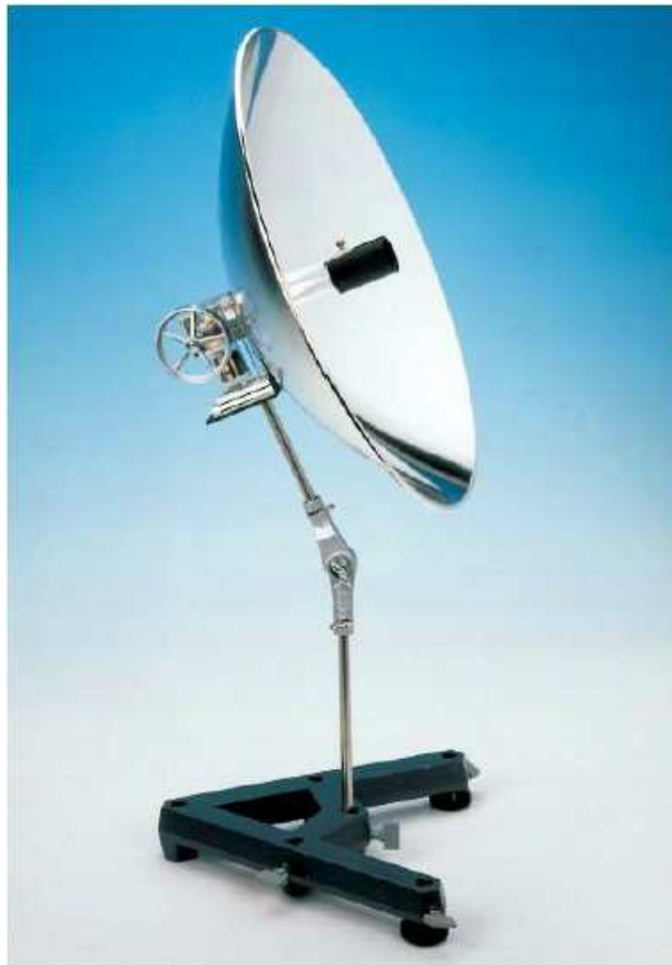
Fig. 9: Stirling engine with accessories for heating by the sun.
