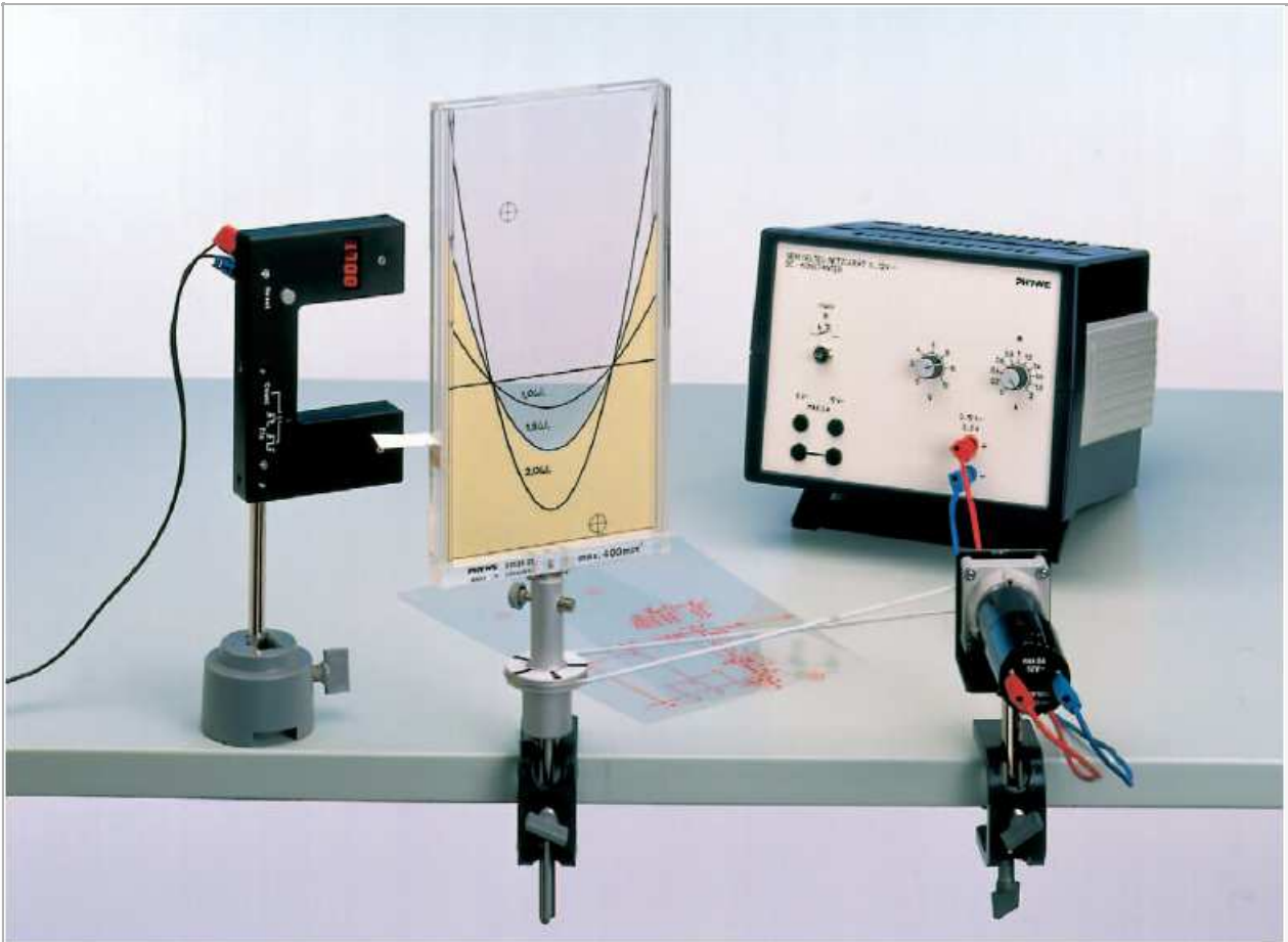
Fig. 1: Experimental set up for determining the parameters of a rotating liquid surface.
