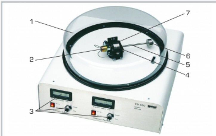
1 protective cover, 2 gyro drive motor, 3 speed displays and adjustment for of the horizontal gyro axis and the vertical precession axis, 4 spinning top flywheel mass, 5 lever, 6 sliding weight, 7 inner frame
