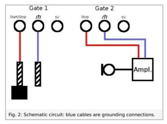
The rod on the barrel base is connected to the Start/Stop jack of Gate 1 at the universal counter. The loose rod with the hole is connected to the Ground jack. Parallel to the input jacks, the capacitor is put on top of both plugs. Thereby, it is ensured that a contact bounce of the rods will not trigger multiple start signals.
