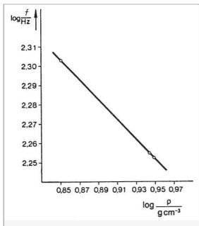
Fig. 5: Relationship between the fundamental frequency f and the density  $\rho$  of the material for a diameter of 0.3 mm, a force of 20 N and a length of 50 cm.
