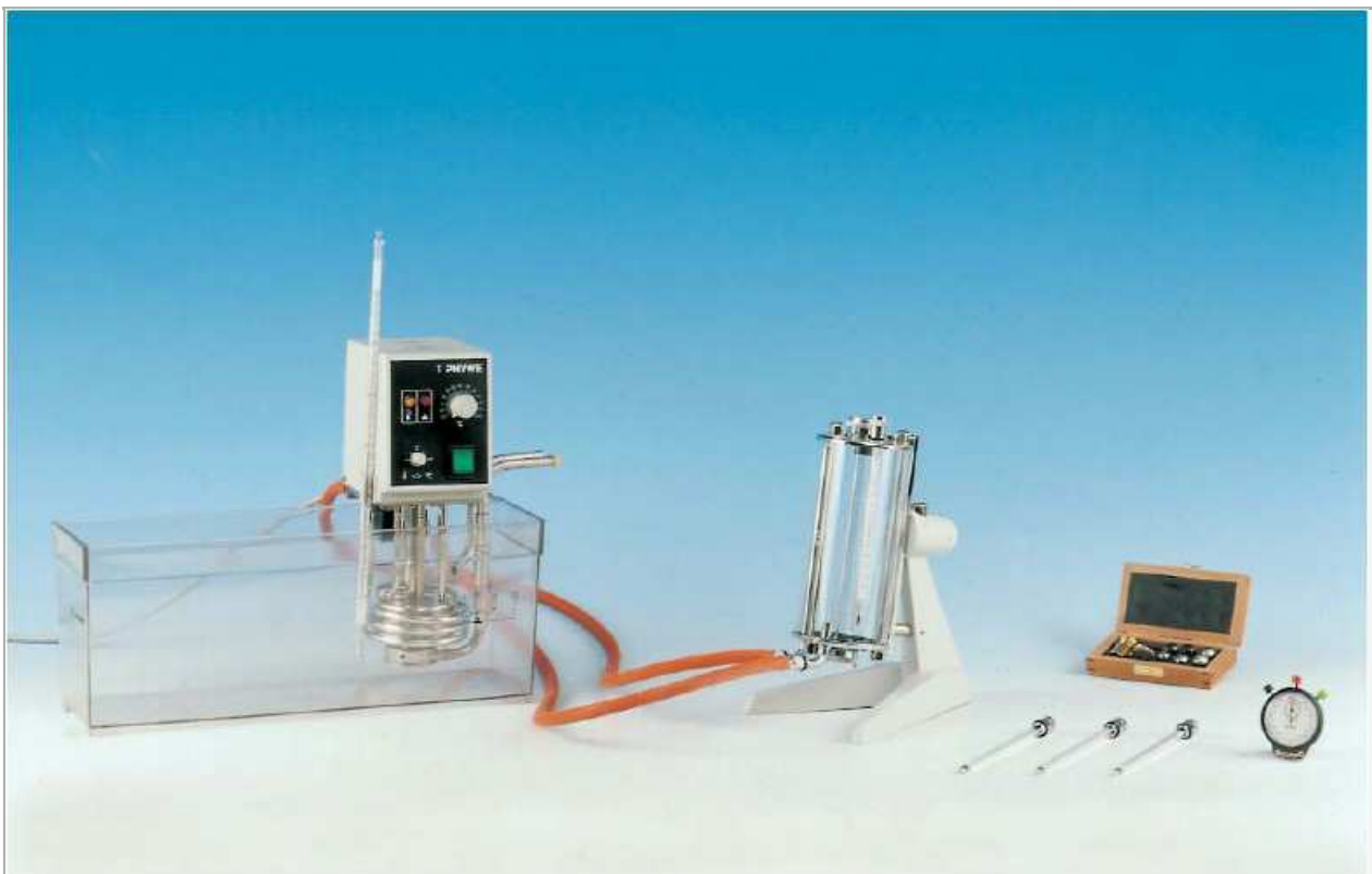
Fig. 1: Experimental set up: Viscosity measurements with the falling ball viscometer.
