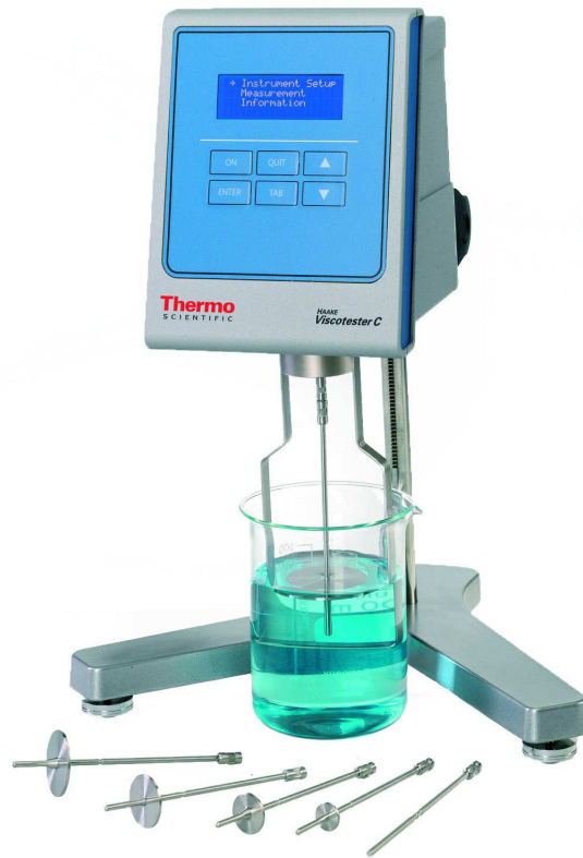
Fig. 1: Experimental set up: Viscosity of Newtonian and non-Newtonian liquids (rotary viscometer).
