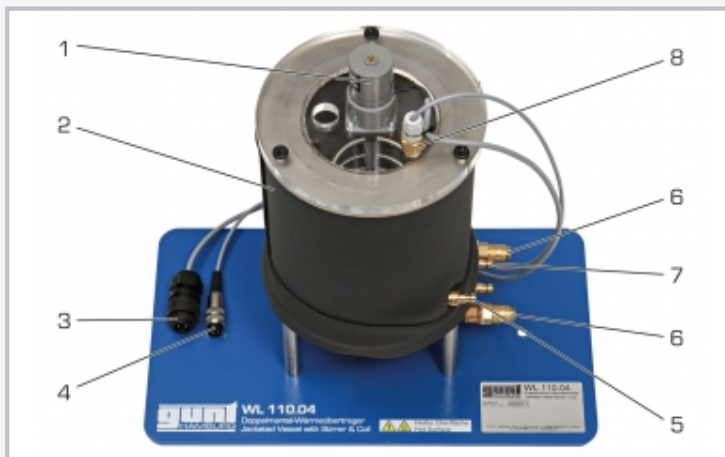
1 stirring machine, 2 stirred tank, 3 stirring machine connection, 4 temperature sensor connection, 5 jacket water connection, 6 water outlet and inlet in stirred tank, 7 coiled tube water connection, 8 temperature sensor
