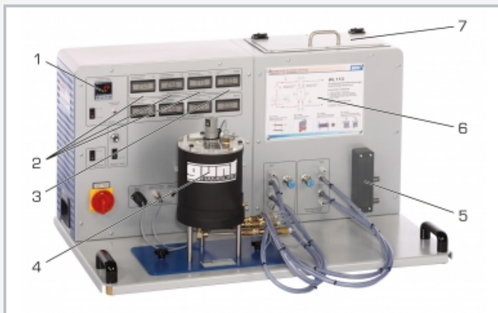
1 temperature controller, 2 temperature displays, 3 flow rate displays, 4 stirred tank with jacketed vessel and coil WL 110.04, 5 cold water circuit connections, 6 process schematic, 7 hot water tank
