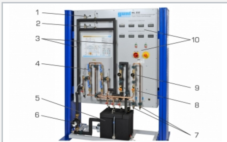
1 bleed valve, 2 temperature sensor, 3 heat exchanger, 4 ball valve for setting the operating mode, 5 tank with heater, 6 pump, 7 water connections, 8 flow meter, 9 valve for setting the flow rate, 10 displays and controls
