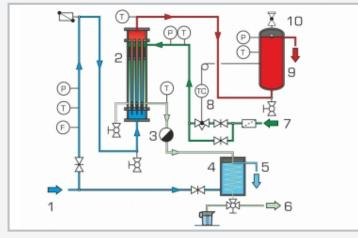
1 cold water inlet, 2 shell & tube heat exchanger, 3 condensate separator, 4 condenser, 5 cold water outlet, 6 condensate extraction, 7 steam inlet, 8 thermostatic valve, 9 hot water extraction, 10 hot water tank with safety valve; P pressure, T temperature, F flow rate, TC thermostat; blue: cold water, red: hot water, green: steam, light green: condensate, light blue: cooling water
