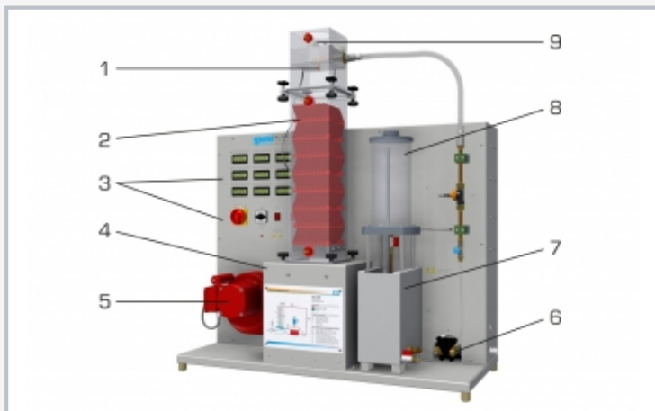
1 nozzle as atomiser, 2 wet deck surface, 3 displays and controls, 4 air chamber, 5 fan with throttle valve, 6 pump, 7 tank with heating, 8 tank for additional water, 9 combined temperature/humidity sensor
