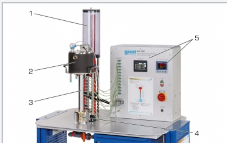
1 raised tank for constant initial pressure, 2 heat source, heater, 3 specimen, 4 water-cooled heat sink, 5 switch cabinet with controller and displays
