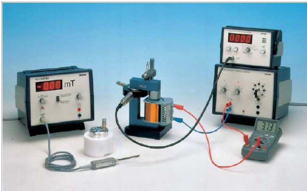
Fig. 1: Experimental set-up for determining inductance from the resonant frequency of an oscillatory circuit.
