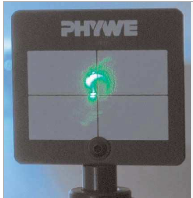
Fig. 7: Bad laser tube alignment
