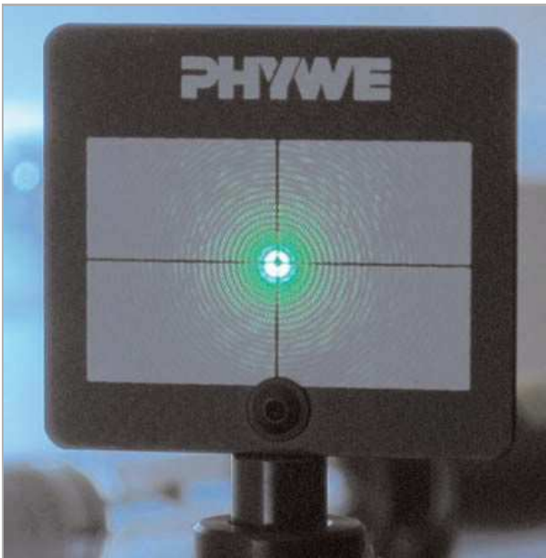
Fig. 6: Good alignment of the adjustment beam
