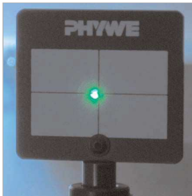
Fig. 8: Good laser tube alignment
