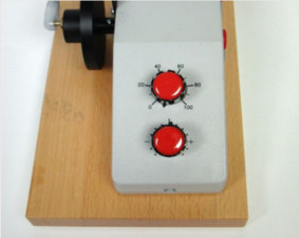
Fig. 5: Control knobs to set the motor potentiometer. Upper knob: "coarse"; lower knob: "fine".
